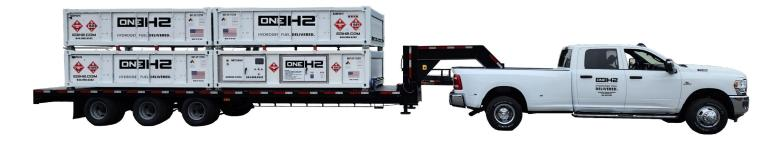
OneH2's 930 bar gas system is designed and manufactured in the USA to meet the most stringent quality standards to safely transport hydrogen fuel on road.
