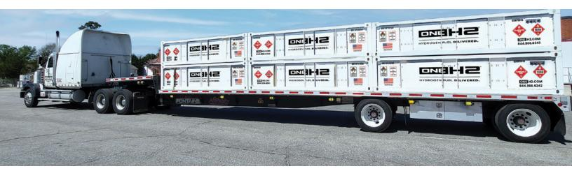
930 Bar Trailers are configured with a modular carrier system. A single carrier consists of three (3) Type IV Cylinders with 80 kg gross capacity of hydrogen each at 13,500 psi.
