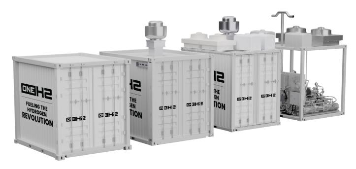
The H-Series design is based On the creation of modules to cover each of the process steps associated with generation of hydrogen gas. The H200 system generates 200 Kg per day of compressed gas to standard SAE J2719 at 7,500 PSIG.
